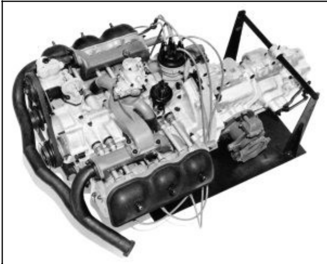
prototype watergekoelde 6 cilinder boxermotor
